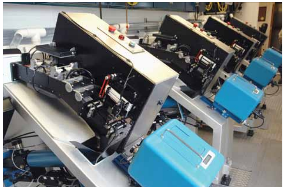
Automated fin-clipping machines mounted in trailers are used to mark young hatchery-raised salmon and steelhead before they are released.
