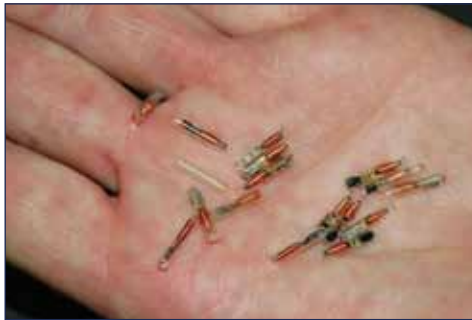
Tiny PIT tags identify fish and their origin.
